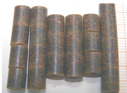
Fig. 3. View of pellets from the mixture of tobacco and lemon balm waste received for parameters of point 8 of the experiment plan ( z_m = 30\% , t_w = 80^\circ\text{C} , l_m = 47\text{ mm} and m_p = 0.9\text{ g} ).
